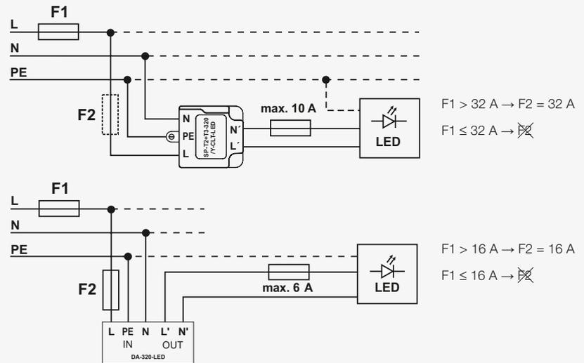
Fig. 10b SPD wired in parallel to the protected equipment
