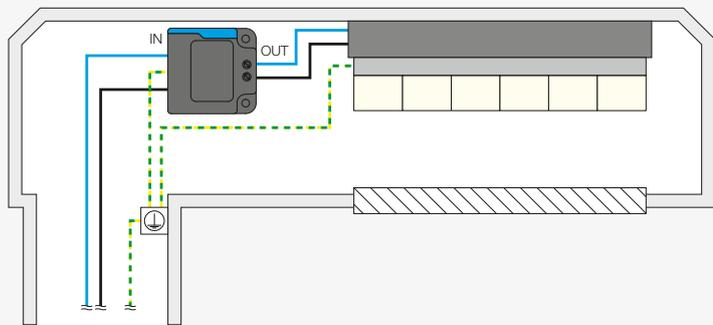
Fig. 14 Example of connecting the SPD to equipment of protection class II
