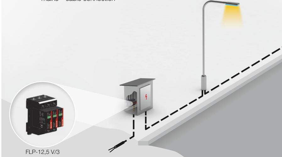
Fig. 2 SPD for lighting circuits installed in a vast building
